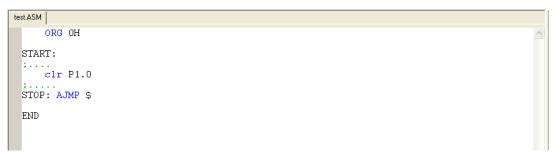
This program changes port pin P1.0 to logic low level. P1.0 is connected to the Green LED on the Training Board (TB-1) so this program will turn on the Green LED if TB-1 is installed. Build the program by clicking the Build button. If the program builds successfully, you will see the following messages on the Output Window:
